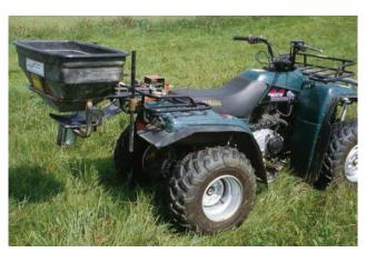
**Figure 6.2.** Spinner-type seeder for frost seeding mounted on an all-terrain vehicle.
